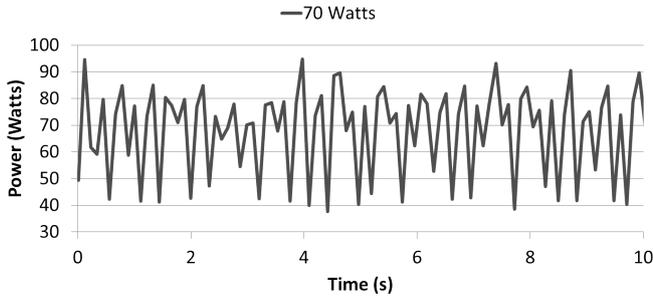
Figure 5: The inherently unstable `bodytrack` application. To increase readability, we show the measurements only for the 70 Watt limit. The other limits exhibit similar oscillations.
